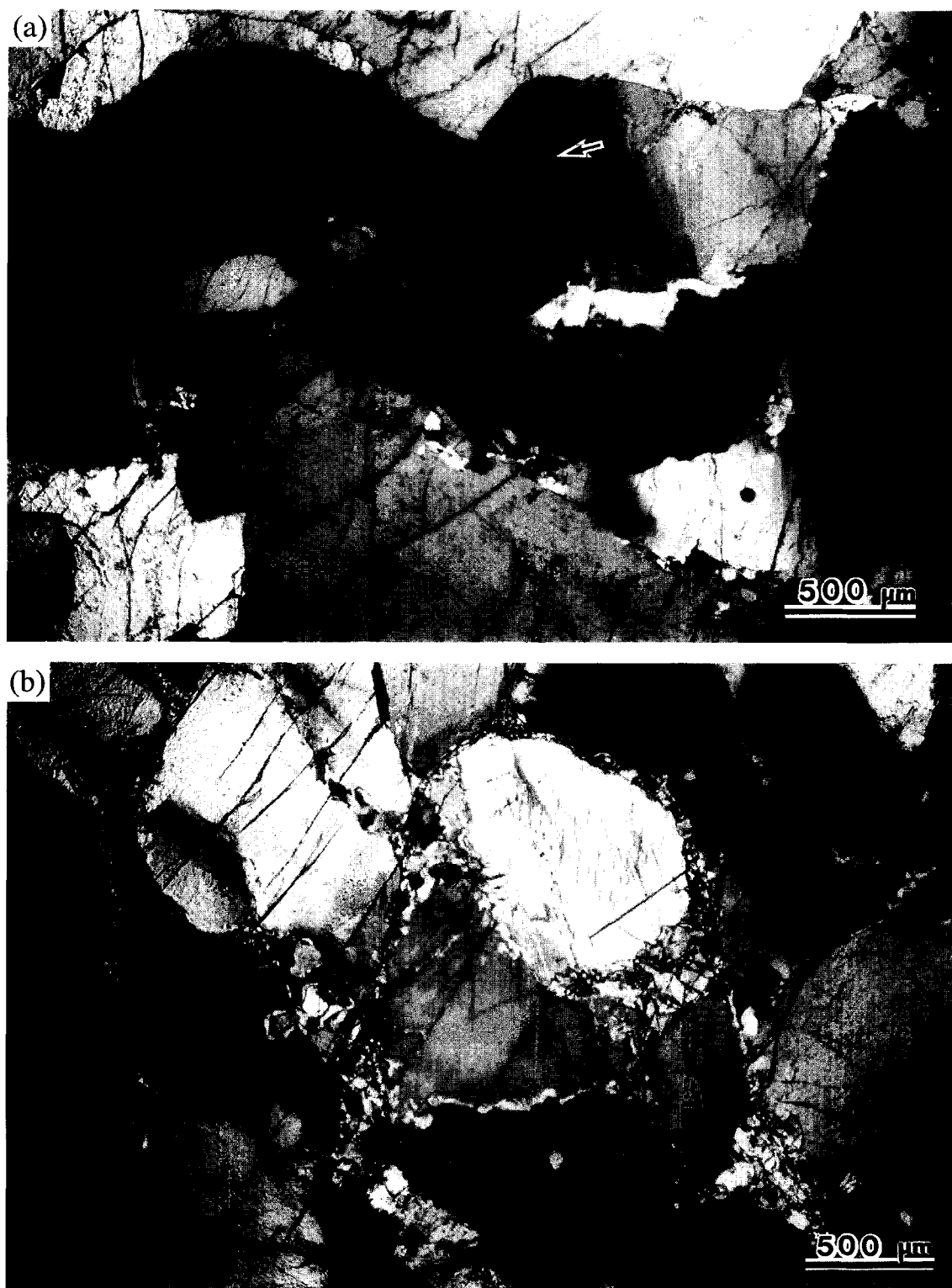
Fig. 3. Optical micrographs of samples (all crossed nicols). (a) Sample BM-11, 70 cm away from pseudotachylyte vein (fault). Very little recrystallization is observed, although evidence of high stress deformation is clear from kink bands in olivine (shown by an arrow). (b) Sample BM-13, 8 cm from the pseudotachylyte vein. The degree of recrystallization is significantly higher than that in a sample further from the pseudotachylyte vein.
